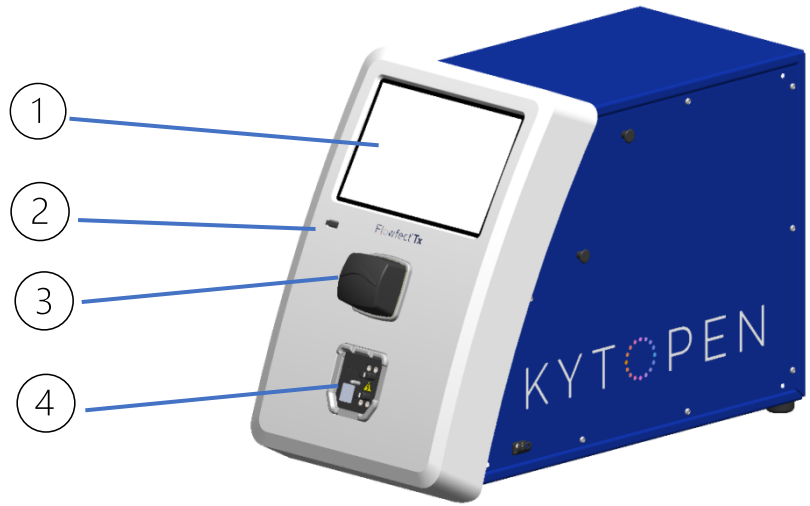
Figure 2: Flowfect ® Tx control unit components
